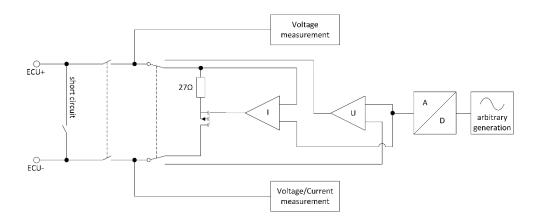
The VT7820 has circuits to simulate either a voltage or a current based sensor. To vary between these two possibilities the signal path will be set by switching the relevant relays.
