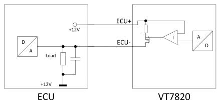
Simulating voltage modulated sensors
